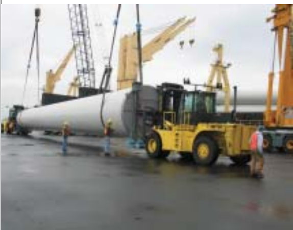
Careful handling and specially designed transporters ensure wind tower sections remain damage-free from ship to storage area.
